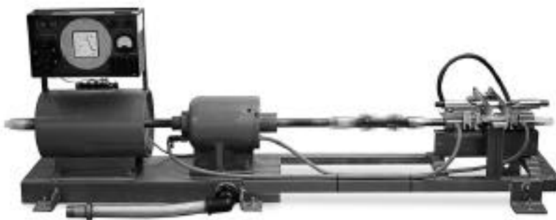
A Dynamic Linear Mass Accelerator (DLMA Linear Engine) working prototype, producing 250 volts at 50 hertz.
